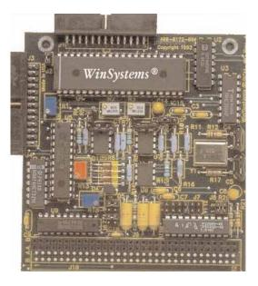
Potentiometers are on the card to permit both gain and offset adjustment.
